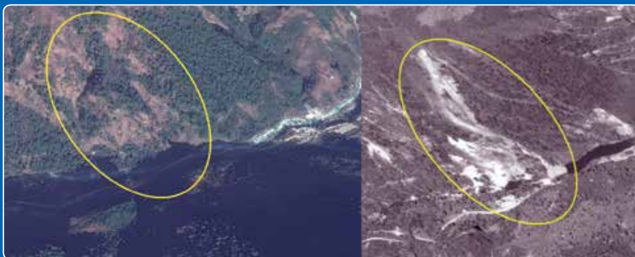
Figure 22: Shallow landslide temporarily blocking the Sun Koshi River about 1 km downstream from Chaku village
