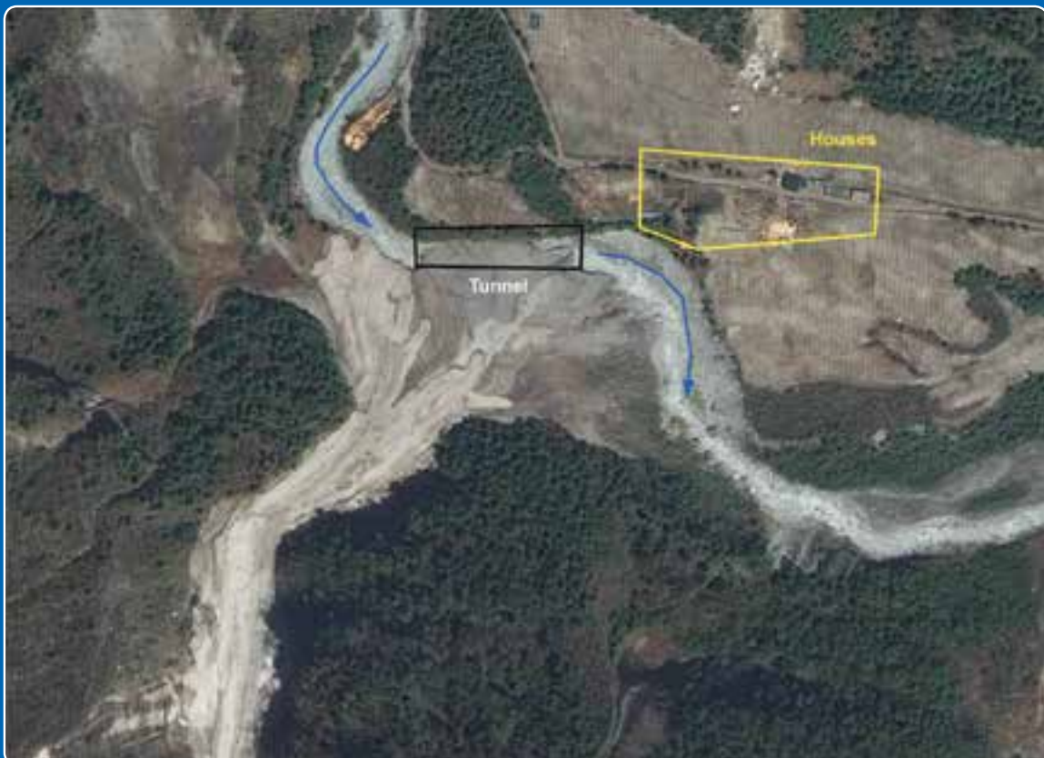
Figure 18: Landslide blocking the Marsyangdi River close to Bhratang village in Manang
